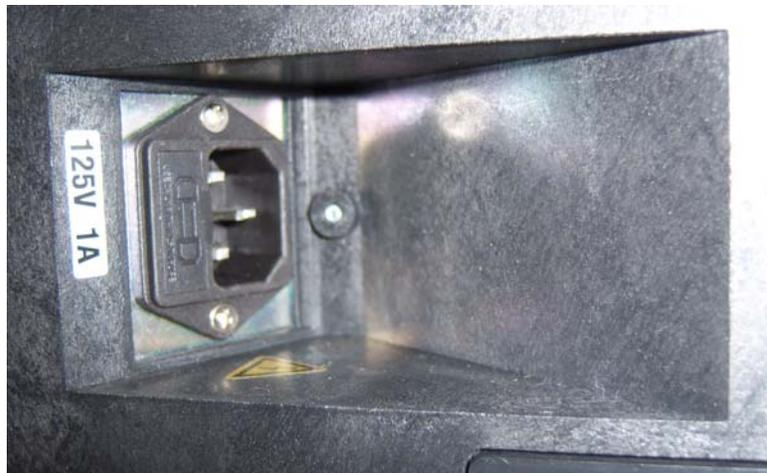
Figure 2-2. AC Plug-in Location on Underside of DC-782
