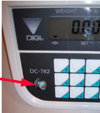
Figure 2-1. Leveling Bubble
